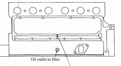
If you are running high pressure engines, drill and tap #10-24 set screw to hold down the distributor and oil pump drive bearing down.
