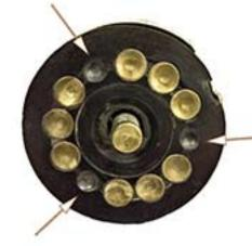
The second problem are the three Black OFF detents. They are .017 deeper resulting to make it harder to move out of the detent. Take a knife and scrap the edge of the hole to tapper edge.
