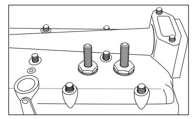
3) Thread the 1/2-13 stud into the spark plug hole adapter until the bottom of the stud is flush with the bottom of the adapter. Thread the adapter/stud assembly into the spark plug hole threads and tighten.
